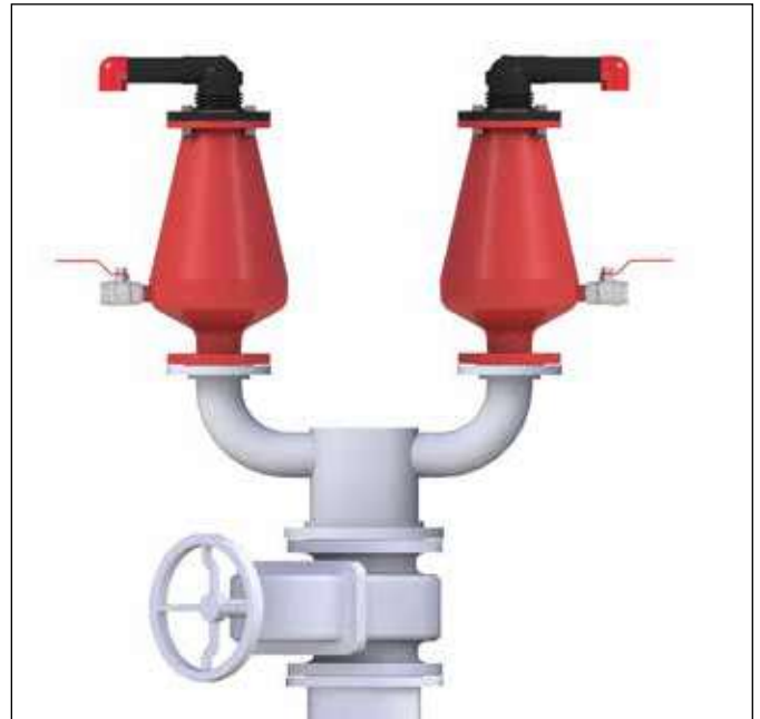
Two Air Valves on a shared Isolating Valve. Air Valves outlets face outward and the Isolating Valve at 45° to Air Valve outlets
