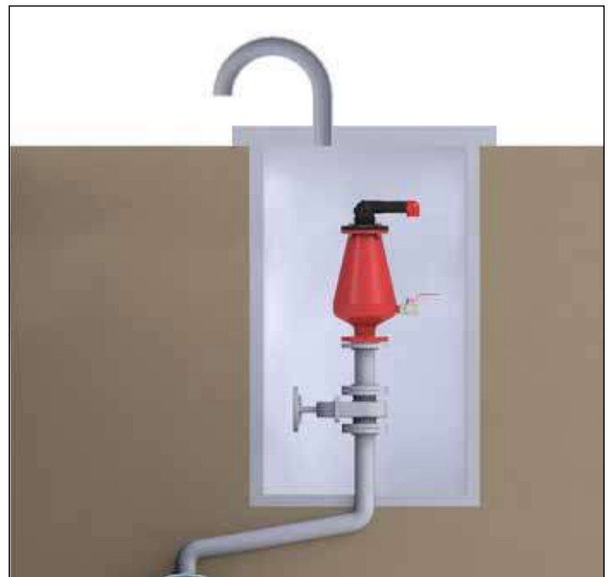
Underground Installations - Underground installations require a venting pipe from the manhole - Use an angular installation to bypass an obstacle directly above the pipeline.
