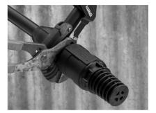
3. Using a pipe wrench or multigrips on the end caps only, further screw the non-return/foot valve into the male thread until tight. Where necessary ensure the male thread is held stationary to avoid it from moving. Do not use pipe wrench or multi-grips on the body of the non-return/foot valve.
