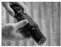
2. Screw the valve onto male thread by hand until firm. Confirm the correct orientation of the valve by checking the water direction arrow is pointing downstream.
