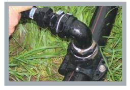
4. When adding additional fittings it is recommended that either a thread sealing paste or thread sealing tape be used on all threaded connections. We recommend LOCTITE 5331.
