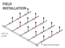
Senninger's Quick Connect Couplings make it easy to disassemble the system in manageable sections.
