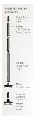
The Inverted Mister is designed for propagation and other low volume misting applications. Its built-in check valve prevents draining immediately following each irrigation session. It also provides consistent system start-up – delivering an instantaneous, highly uniform distribution, ideal for short-cycle applications.
