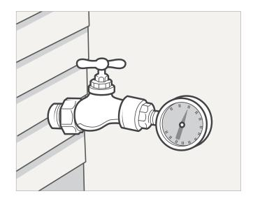
**Figure 1:** To check water pressure, attach a pressure gauge to the outside faucet nearest the water meter. A pressure gauge can be obtained from your local Hunter dealer.
