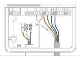
Use colour-coded irrigation wire to connect the valves to the controller. You will need one wire for each valve, plus one common wire.
