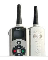
The Hunter ROAM Remote Control Kit saves time during installation and routine system maintenance. The receiver (right) plugs into the Controller Connection Kit and the transmitter (left) activates the sprinklers within a 300 m range. The user can manually run any zone without resetting the controller. Compatible with X-Core, X2, Pro-C, ICC2, and HPC controllers.
