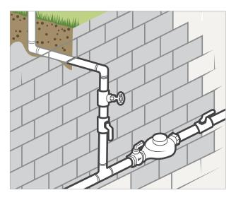
**P.O.C. Freezing Climate:** If the P.O.C. is in the basement, install a boiler drain immediately after the gate valve to drain the system before the first big freeze.
