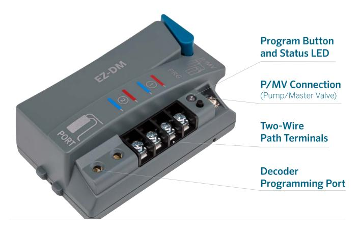
Plug in the EZ-DM two-wire output module to enable up to 54 stations of irrigation, plus a master valve, on a single pair of wires. Then simply place EZ Decoders at each valve!
