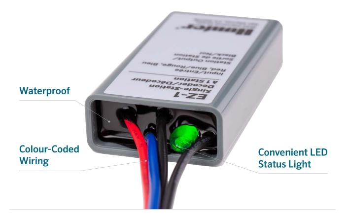
EZ Decoders are small, waterproof, and come with colour-coded wiring and a convenient LED status light. They do not require special wire or connectors to function. Better yet, the system can coexist with conventional output modules, allowing hybrid functionality of both directwired valves and decoder operations in the same controller. This technology also permits simple conversion of a conventionally wired system to two-wire using the existing wiring bundle. It's that easy!
