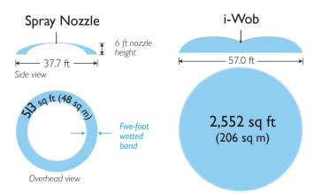
In this example, the i-Wob is spreading the same amount of water over an area five times greater than the area covered by the spray nozzle. Nozzles are at 20 psi (1.38 bar) and at 6 ft (1.83 m) in height, using an 11/32 inch (8.73 mm) nozzle, with a flow of 15.39 gpm (3495 L/hr) in no wind conditions.
