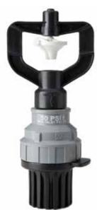
Flow control nozzles (10FC) are an excellent low cost option when system pressure ranges between 25-50 PSI (1.7-3.4 BAR). When system pressure differences are more extreme the Nelson Mini Regulator or Mini Regulator Drain Check are ideal products.
