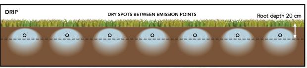
MP Rotators outperform landscape dripline installed under turf or landscape beds. Driplines apply water at point locations that result in uneven water distribution and require overwatering at the emission point.
