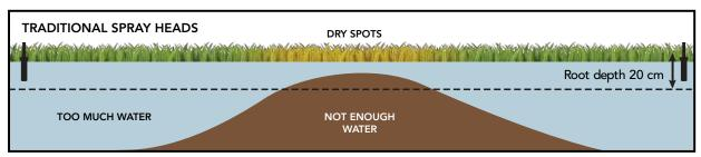
**50% EFFICIENT** Water is dispersed at 40.6 mm per hour causing flooding, which leads to runoff.
