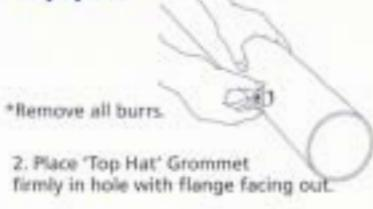
2. Place 'Top Hat' Grommet firmly in hole with flange facing out.
