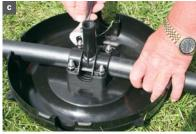
Select the Riser to suit your sprinkler size. Ensure fastening nuts are tightened evenly. Fit O-ring seal to sprinkler riser, locate riser spigot into hole in pipe and fasten the cross tee anchor.
