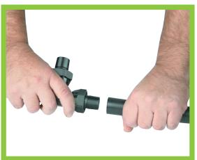
**2** Ensure the nut is fully wound back onto the body of the fitting. Push the pipe onto the fitting and as far as possible into the nut.
